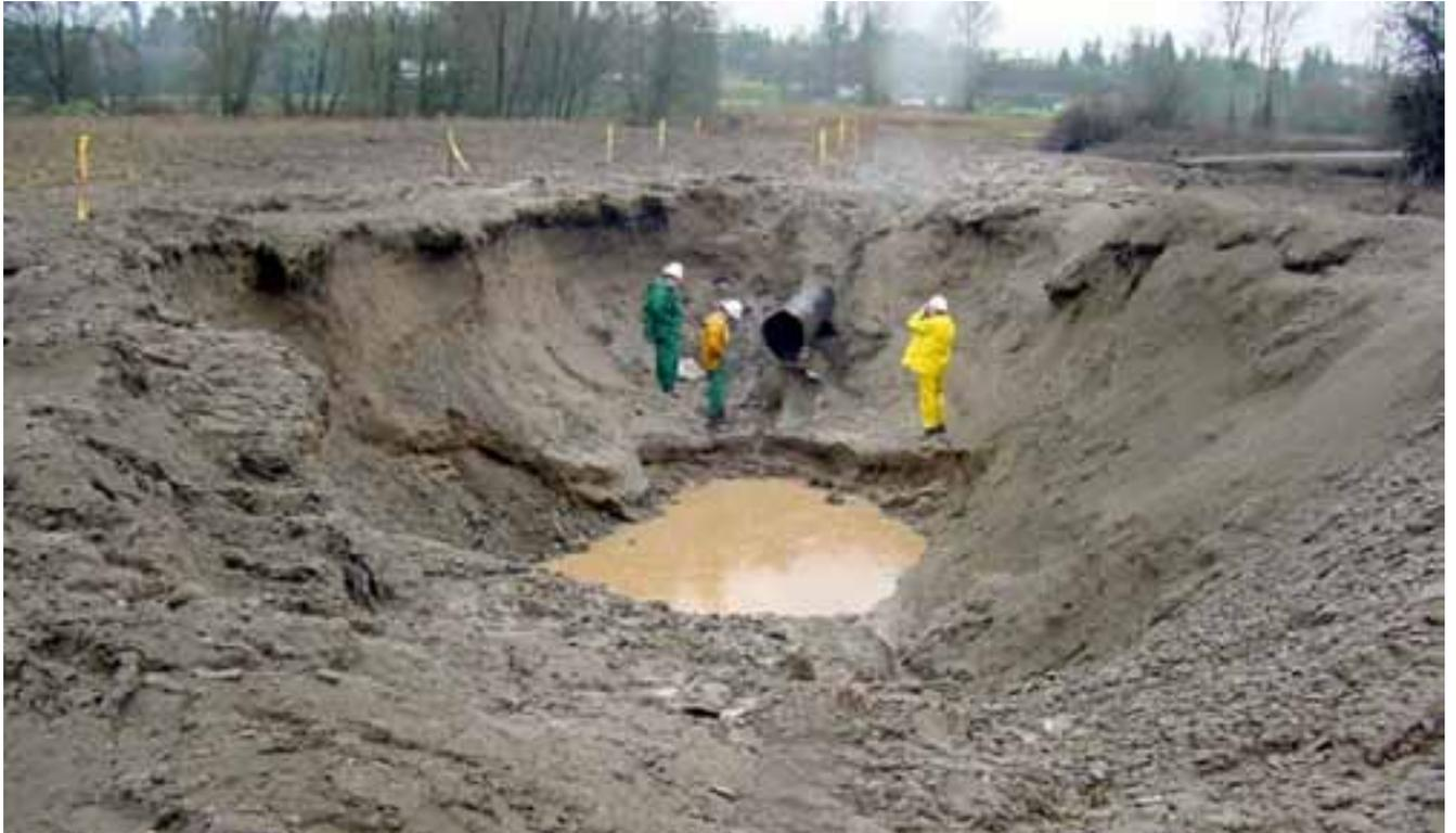
Failure of natural gas transmission pipeline. In this incident there was no explosion or fire, the crater was created by the pressure of the gas coming out of the pipeline. Note how far the pipe in the upper right corner was thrown.
